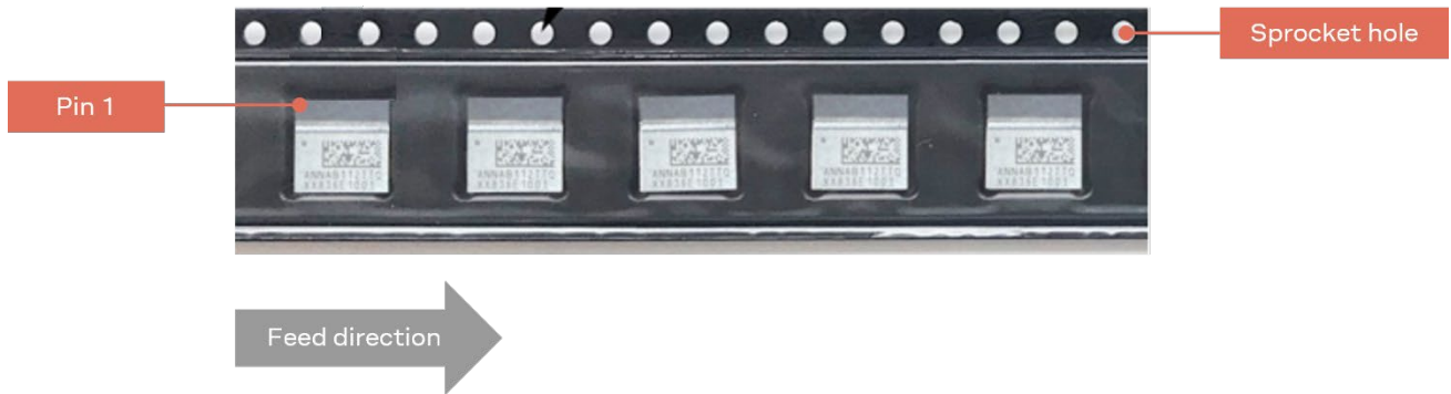
Figure 6: Orientation of ANNA-B4 modules on tape
