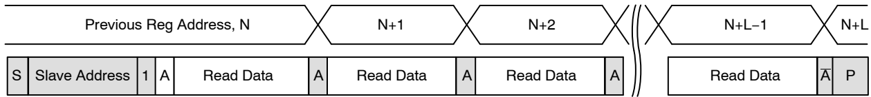
Figure 37. Sequential READ, Start from Current Location
