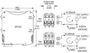
OUTPUT "C" TERMINALS ARE USED FOR OPTIONAL "SOURCING" LOOP WIRING TERMINATION (SEE USER MANUAL)
