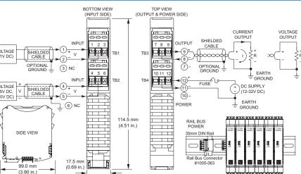
Multi-range ±1V, ±5V, or ±10V input ◆ Universal current/voltage output ◆ 12-32V DC local/bus power
