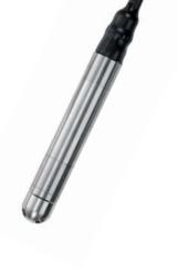
The ILTS is designed for use in continuous submersion in liquids such as water, oil and fuels. The probe uses the latest piezoresistive media-isolated silicon sensing technology and a stainless steel diaphragm. Housed within a 316L stainless steel, or high grade Duplex stainless steel housing, this submersible transmitter is the ideal product for hydrostatic level measurement where temperature is also a critical part of
