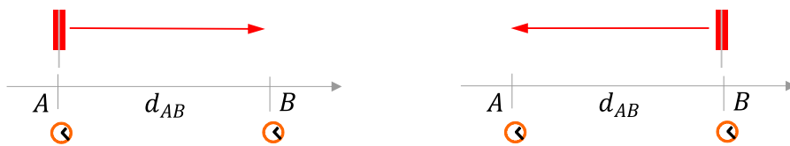
Figure 31: The effect on relative timing of uncertainty in the base station location. This uncertainty is mitigated by using the Timing Advance information from the serving cell.
