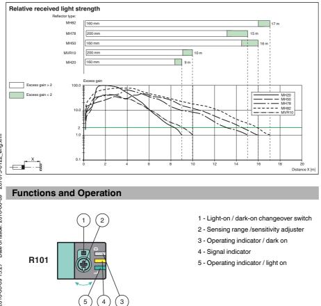
To unlock the adjustment functions turn the sensing range adjuster for more than 180 degrees.
