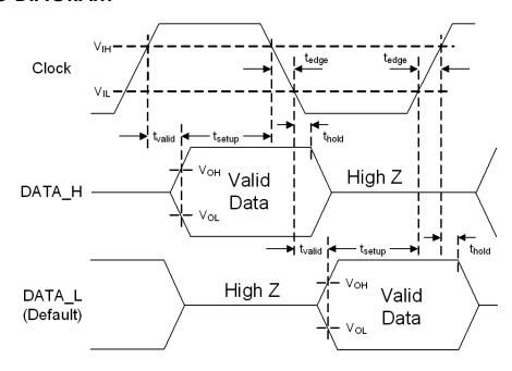
$$T_{clock}/2 = T_{edge} + T_{valid} + T_{setup}$$
