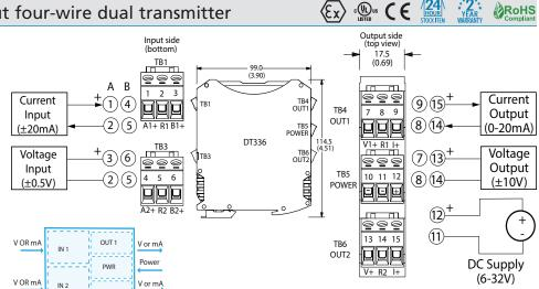
Dual channels ◆ ±20mA, ±500mV inputs ◆ 0-20mA, ±10V outputs ◆ 6-32V DC local/bus power
