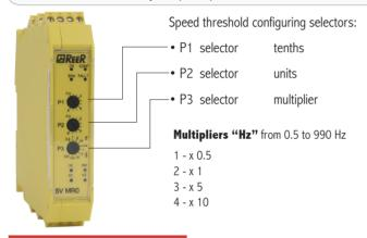
P1 and P2 selectors allow to set numeric values from 01 to 99. P2 selector allows to set a multiplier to apply to the numeric value obtained with the first two. The multiplier can be set in "Hz" or in "rpm" (round per minute). Note: Only when the proximities switches sensor show a single pulse per turn, the value in "rpm" corresponds to the value in "ipm" (pulse per minute).
