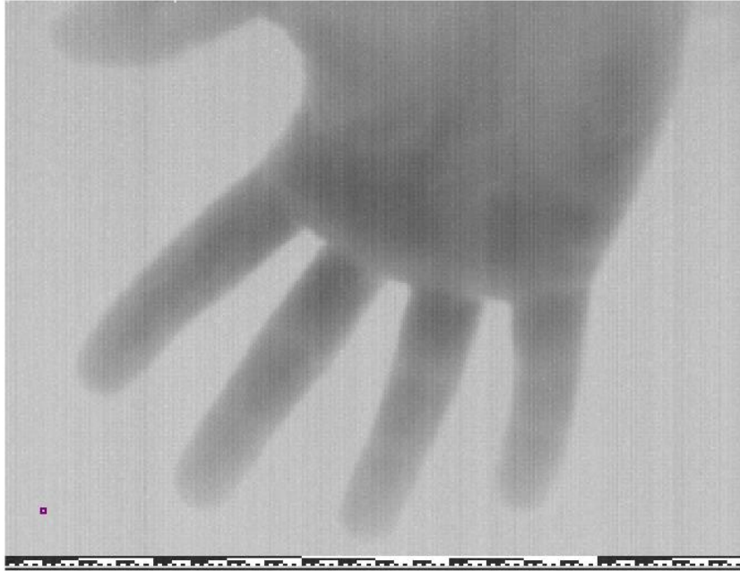
Figure 8: Raw tap A phase180 image of a hand with the test rows enabled
