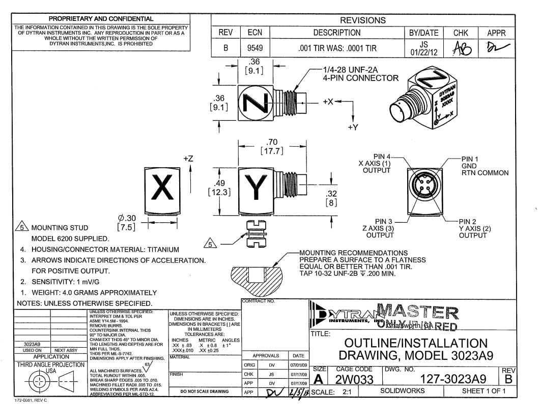
Model Number DOC NO PERFORMANCE SPECIFICATIONS 3023A9 PS3023A9 TRIAXIAL IEPE ACCELEROMETER REV F, ECN 15645, 03/16/20
